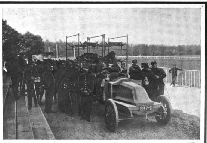
Taxicab transformed into ambulance with eight stretchers
